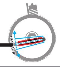
Front kick-up is used to adjust the amount of weight transfer to the front when the vehicle is off-throttle or under braking. Changing the front kick up angle also changes the caster angle (see Caster section).
