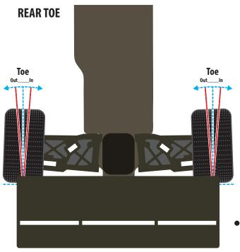
Toe in and toe out are terms used to describe the angle in which the wheels point when looking down at them from the top of the vehicle. Toe is used to stabilize the vehicle at the expense of traction. Front wheels can be toed in or out to suit various situations. Rear wheels should only have varying degrees of toe in.
