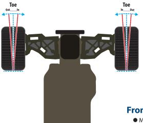
Toe in and toe out are terms used to describe the angle in which the wheels point when looking down at them from the top of the vehicle. Toe is used to stabilize the vehicle at the expense of traction. Front wheels can be toed in or out to suit various situations. Rear wheels should only have varying degrees of toe in
