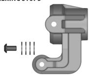
Steering stops simply limit the amount of steering travel and are more accurate at accomplishing this than radio adjustments due to the fact that they are finite. If you set up your end points travel adjustments via your radio, the steering can still travel beyond this in corners when the force of the vehicle can push the servo saver beyond the radio setting.
