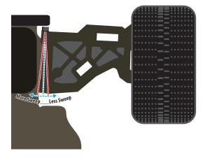
The purpose of sweeping the arm forward or backward is mostly to sweep the driveshafts forward or backward. When the driveshafts are angled it changes how the car reacts on and off power.
