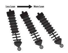
You can manipulate the handling characteristics of the vehicle by changing the shock mounting position. Leaning the shocks at different angles and moving the shock closer or further from the centerline of the vehicle will have different effects on handling.
