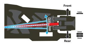
Changes to wheelbase can have a dramatic effect on the handling of your vehicle, since it adjusts the distribution of weight on the rear wheels, which adjusts traction. By shortening the wheelbase at the rear of the vehicle, your placing more weight over the rear wheels, which results in more rear traction). By lengthening the wheelbase, the vehicle feels more stable and the longer vehicle handles bumpy section easier.
